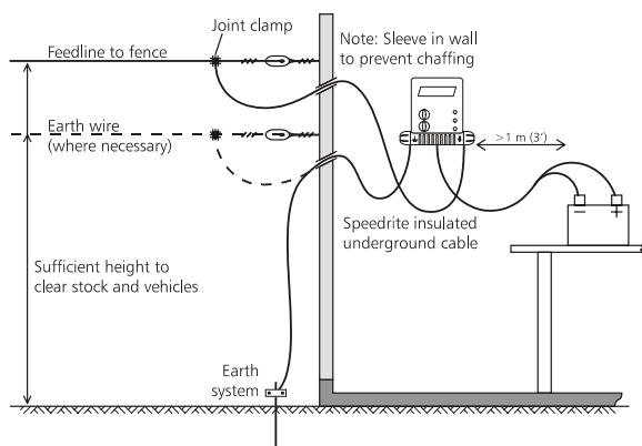
For interior installations, make sure the energizer and battery are level. Mount them above floor level and out of reach of children.
