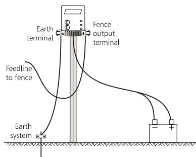
For exterior installations, ensure that the energizer is protected from animals and the environment. If necessary, house the energizer in a protective box. Consider site access, proximity to a suitable area for earthing and whether the energizer is safe from human interference. Try to position the energizer as near as possible to the centre of the electric fence.
